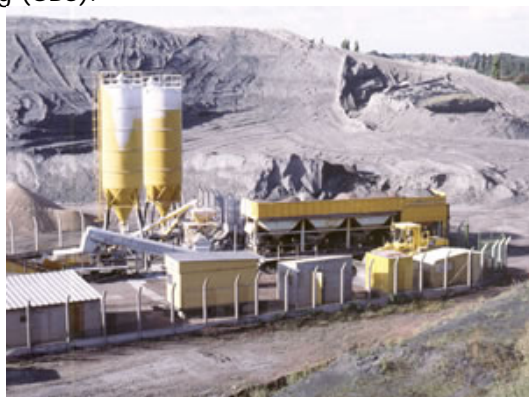
Production facilities of HBM mixtures.
